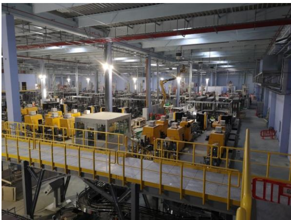
Image 3: In the "cold end" of the plant, once moulded, the containers pass through the annealing furnaces and are then subjected to quality tests.
