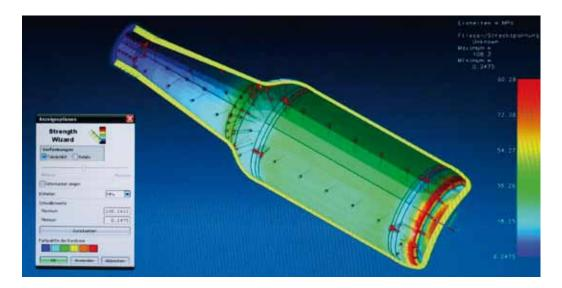
Finite element analysis reveals where the stresses are greatest: points under particular stress are coloured red.
