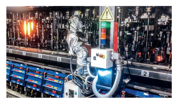
One of the machine operator's main jobs during production is to apply an oil graphite paste evenly and precisely onto the blank moulds and opening and closing mechanisms at regular intervals using a brush-like applicator. This is absolutely essential for ensuring the quality of individual articles. Since every machine operator has their own working style, one 24-hour production cycle can result in a considerable amount of variety.
